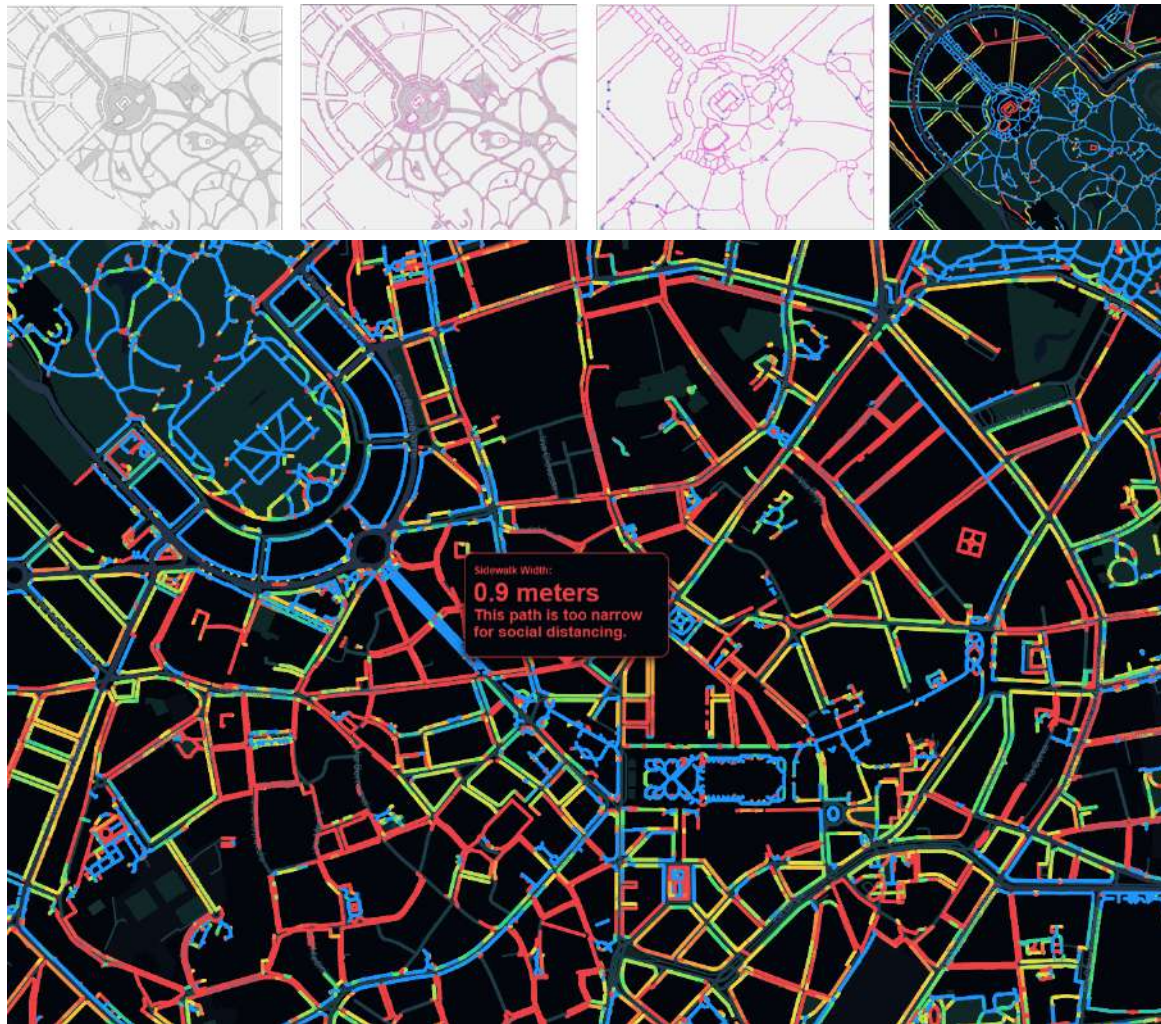
Fig. 6 A screenshot from the interactive map showing sidewalks widths in Milan and highlighting the critical areas where physical distancing cannot be respected: very difficult (less than 2.4 m), highlighted in red; somehow doable (between 2.4 and 3.3m), in yellow; doable (between 3.3 and 4.2 m), in green; easy (more than 4.2 m), in blue.
