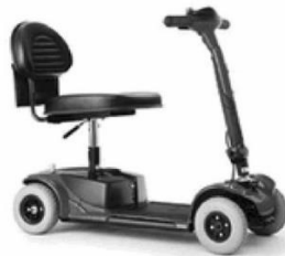
Fig.4 According to the EU Regulation 718/2009, this four-wheeled device is a "special type of a vehicle for the transport of persons" which is not specially designed for the transport of disabled persons and has no special features to alleviate a disability (source: Official Journal of the European Union L205 of 7 August 2009)
