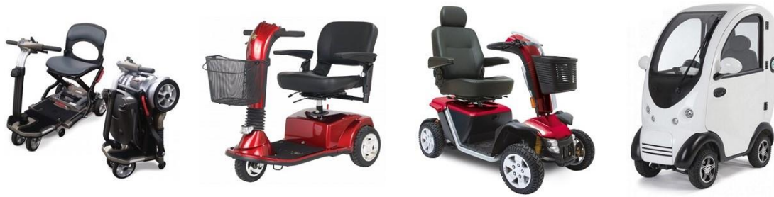
Fig.1 The various types of mobility scooters: portable, three-wheel, four-wheel, and cabin (source: Officine Ortopediche S.r.l. )
