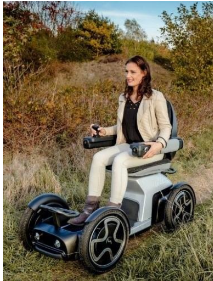
Fig.7 This device should be classified as mobility scooter because of the presence of a steerable front axle, even if it steers with a joystick (source: scoozy.nl ; photographer: Jorrit Lousberg )
